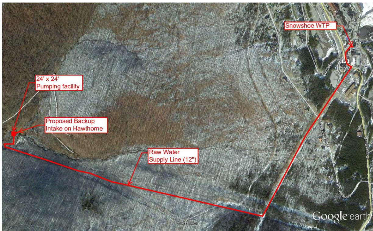
Figure 3. Cheat Mountain Water Backup Intake Conceptual Drawing
