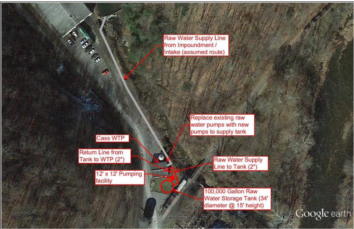
Figure 3. Cass PWS Raw Water Storage Conceptual Drawing
