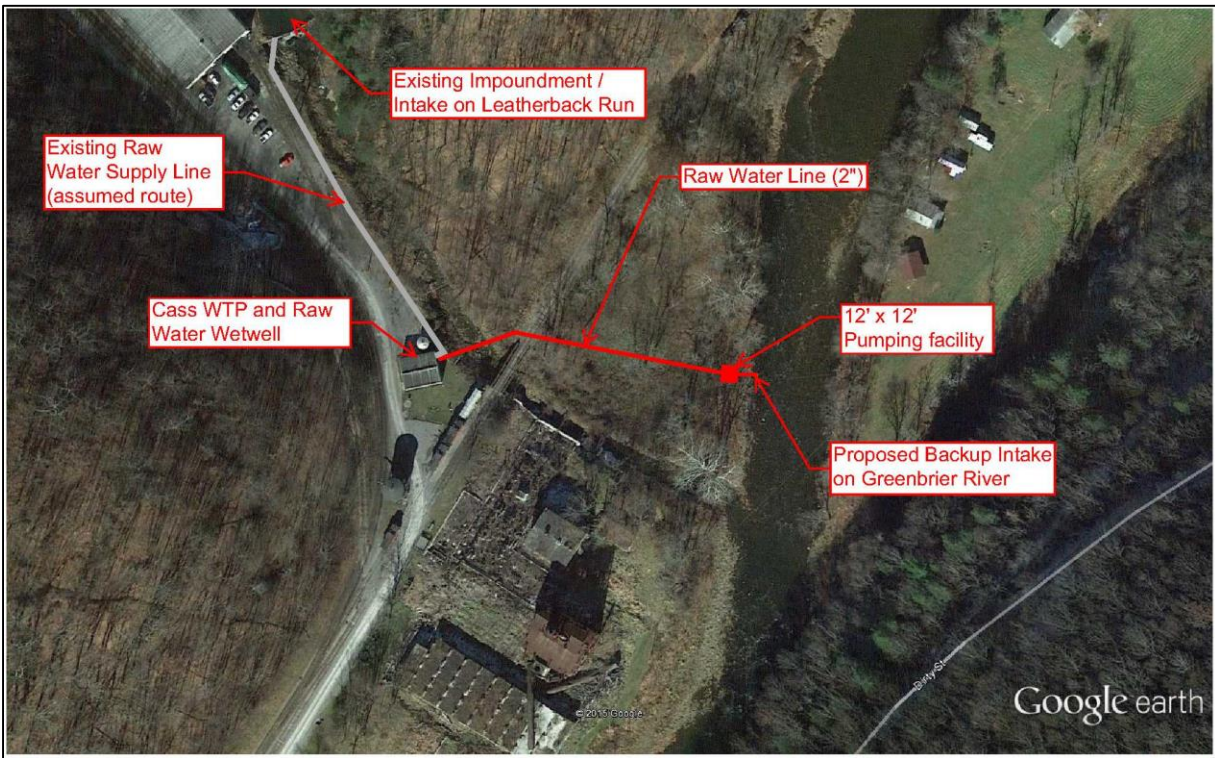
Figure 2. Cass PWS Backup Intake Conceptual Drawing
